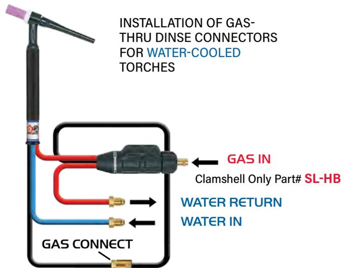
*For a quick disconnect installed on your water lines add "QD" to the end of the dinse part number.*
